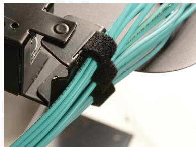
Small Diameter Bundles AOC's thin diameter allow for smaller bundles which promotes better airflow.
