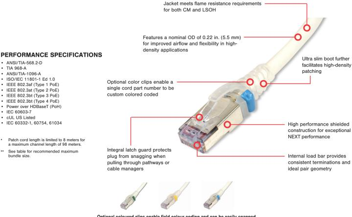
Optional coloured clips enable field colour coding and can be easily snapped into place without having to disconnect cords
