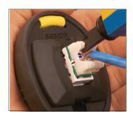
**Termination**Siemon's Palm Guard with MAX insert (p/n: PG-MX6) assists in securing outlet during termination.
