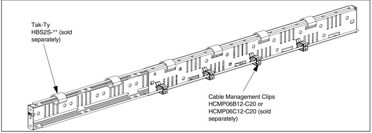
It is possible to hold any vendor's cable or cable transition to front & rear brackets with two alternative methodologies: Tak-Ty (hook-n-loop cable tie) and harness clip fasteners (cable management clips). Cables can be secured to the left or right mounting brackets or strain relief bar with 0.75 inch wide Tak-Ty (hook-n-loop cable ties) which mount through the horizontal slits or cable management clips. The cable management clips mount into 0.25 inch diameter holes located on the brackets.
