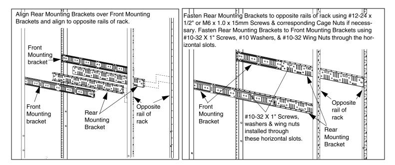
NOTE: If installing strain relief bar from FLEX-CM-1UBKIT, do not completely tighten wing nuts at this time.
