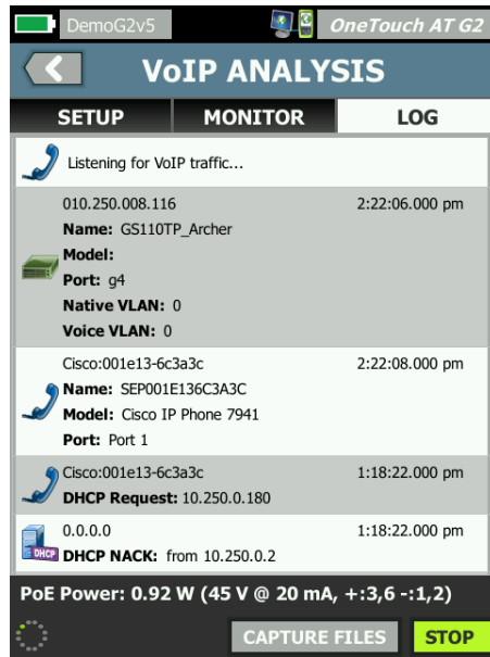
Figure 18. VoIP Analysis shows the entire call setup process as well as quality of the VoIP call in each direction
