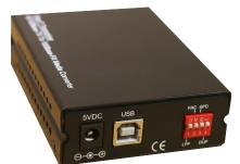
These very simple and easy-to-install Ethernet media converters are ideal for extending Ethernet networks over fibre. Suitable for small office to enterprise applications, they can be used as standalone units for connecting remote locations or they can be fitted into a rack mountable frame suitable for Comms room environments.
