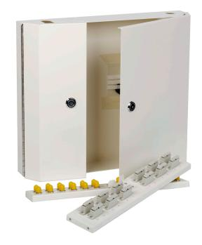
The wall boxes can be supplied with SC duplex, LC quad, ST or FC style adapters. They can be configured for Singlemode or Multimode applications and are available fully loaded, partially loaded or unloaded as required. They are supplied complete with 1 x PG11 gland and 4 x Kurly Loks for cable management.
